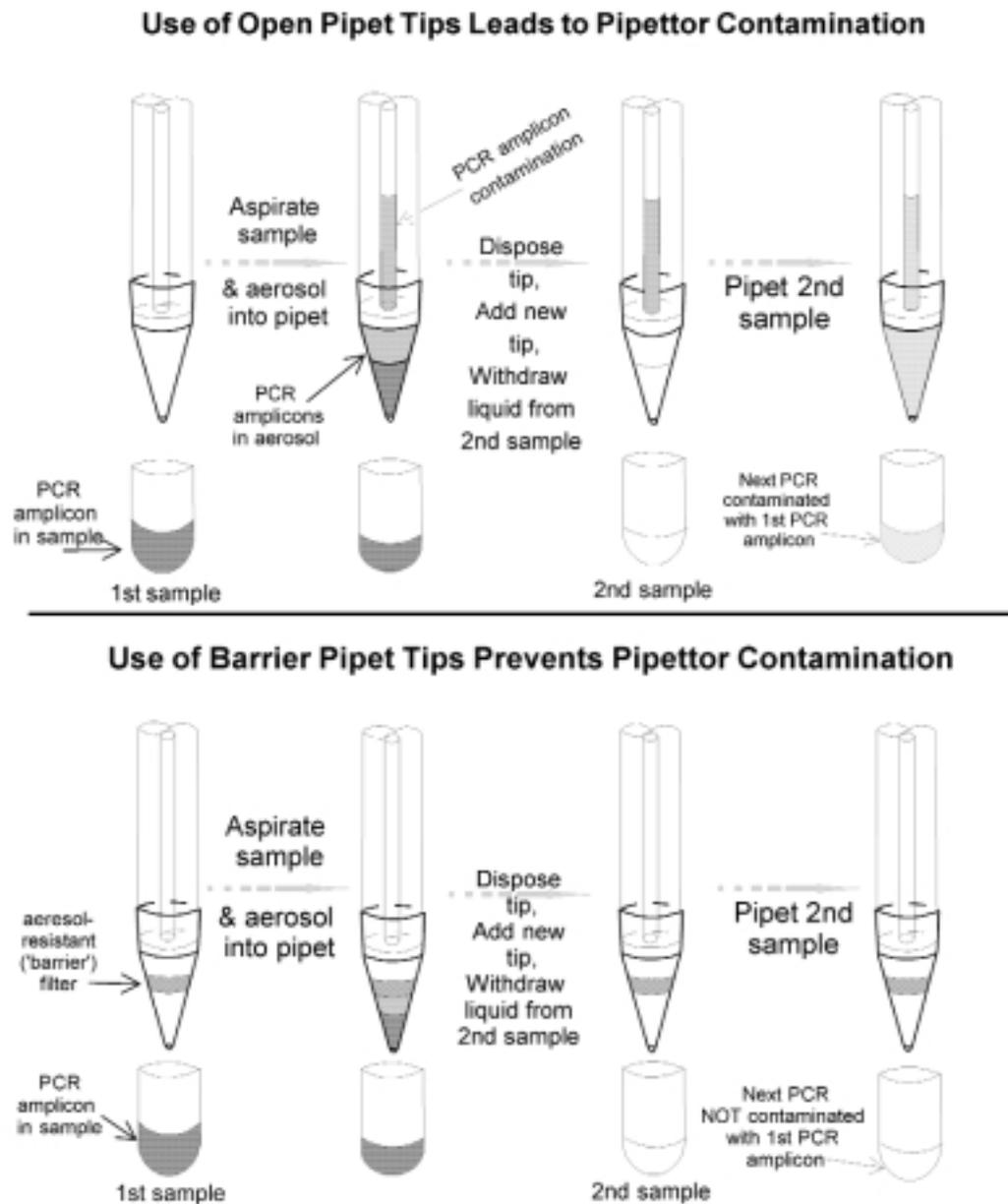
FIGURE 3. Use of barrier tips to prevent amplicon contamination in the PCR laboratory.
